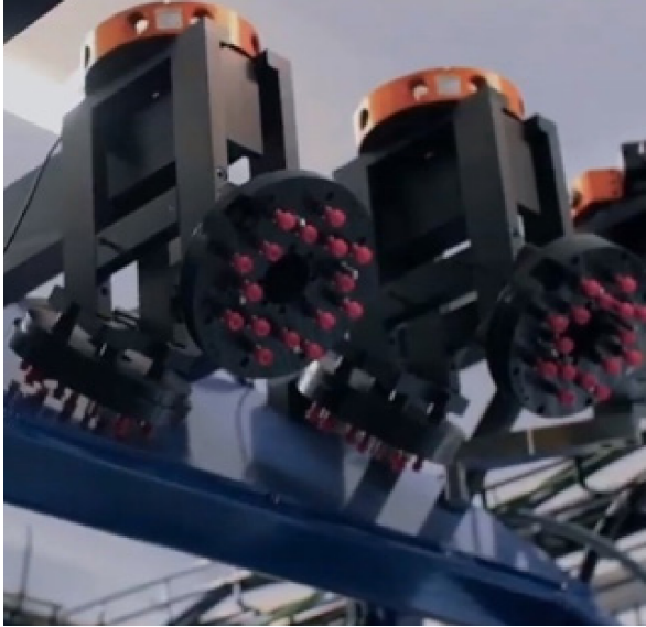
ATI tool changers with vacuum tools for plastic parts
